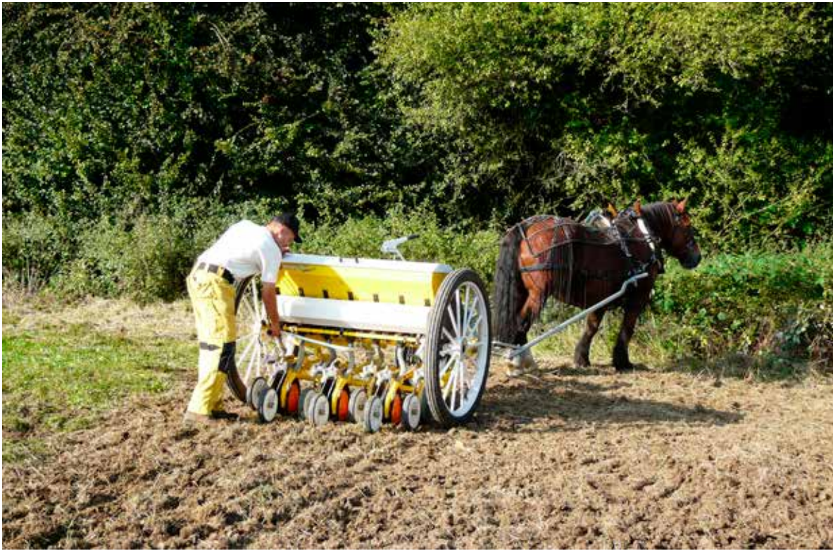
Lifting the coulters and shutting off the seeding mechanism by the rear lever before the turning maneuver at the headland (Photo Cathy Laroche 2015)
